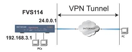
Figure 5-1: Client-to-gateway VPN tunnel
